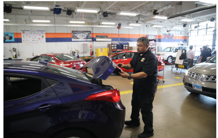
A Cook County Sheriff's Department mechanic replaces a car lamp at Morton College.
